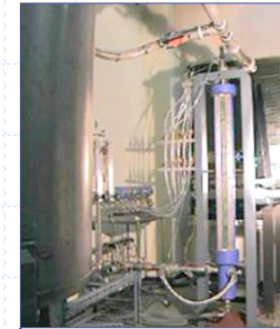
Wire Spacer Pressure Drop Experimental Facility
